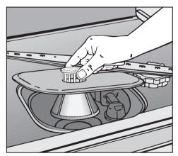
Lift the filter combination out of the machine. Remove any coarse particles and rinse the filter under running water. Use a nylon brush if necessary.
